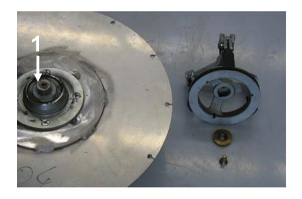
Remove the feather key of the drive shaft. Unscrew the countersunk bolts from the bearing flange. Use an extracting tool to remove the bearing flange from the shaft.
