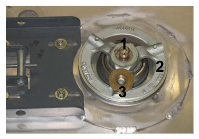
Use an extracting tool to remove the belt pulley (2) from the shaft.
